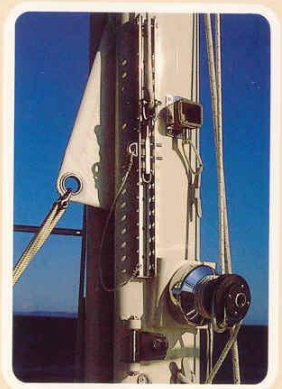
the mainsail halyard tightening system
