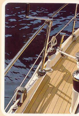
the handle-operated jib sheet traveler
