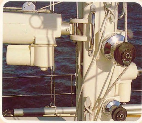
the electric roller furling mainsail and electric clew
