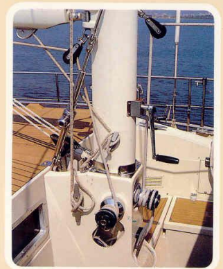
the mizzen mast foot
