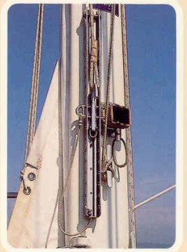
the mainsail halyard tightening system
