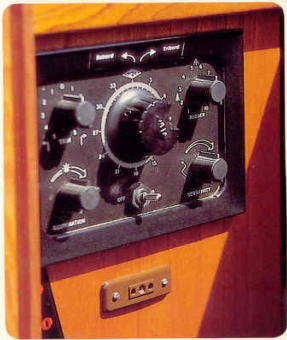
autopilot control panel
