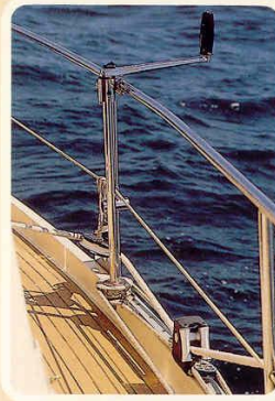
the handle-operated jib sheet traveler
